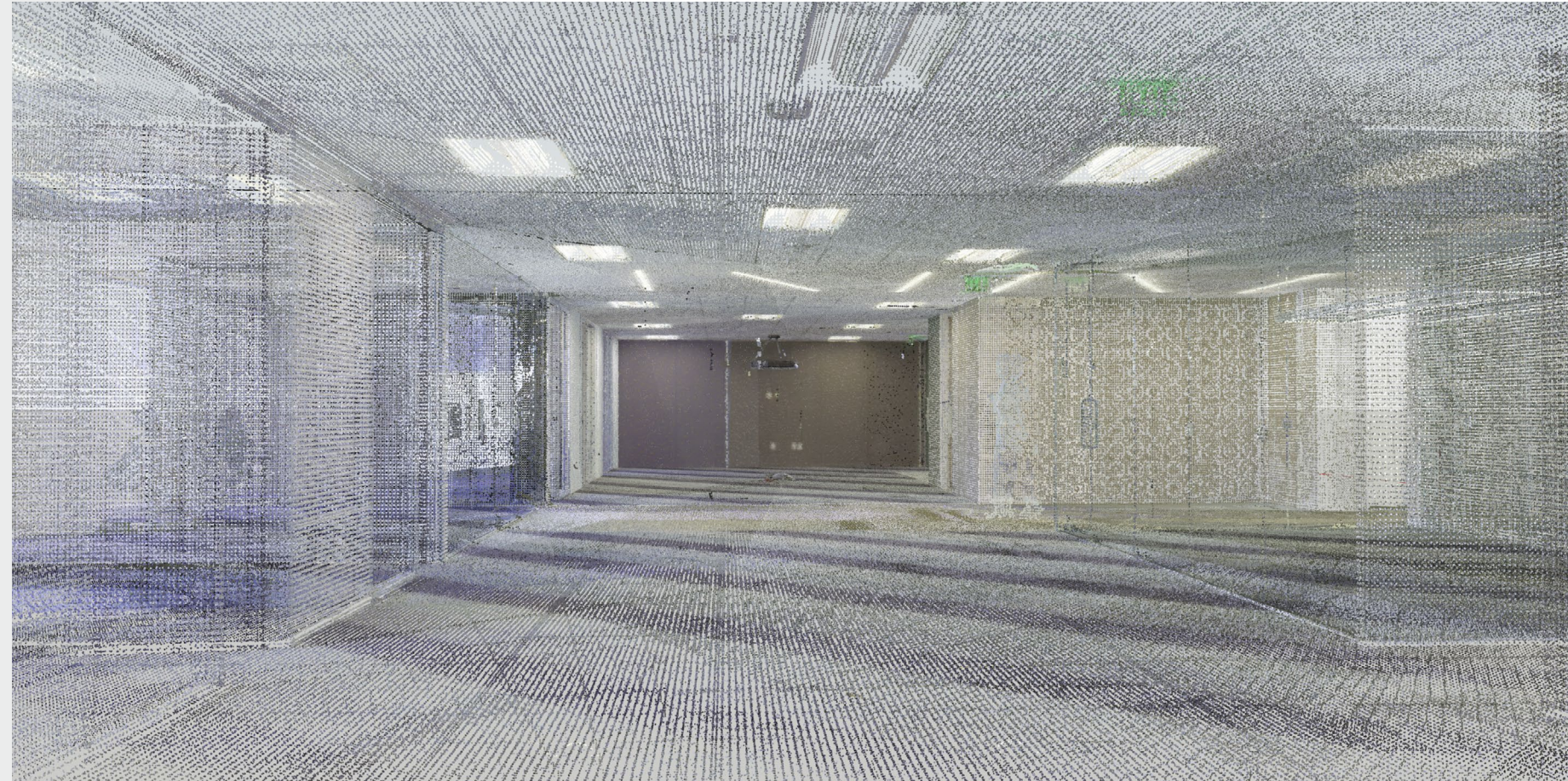
Point cloud data imported into 3D software.
