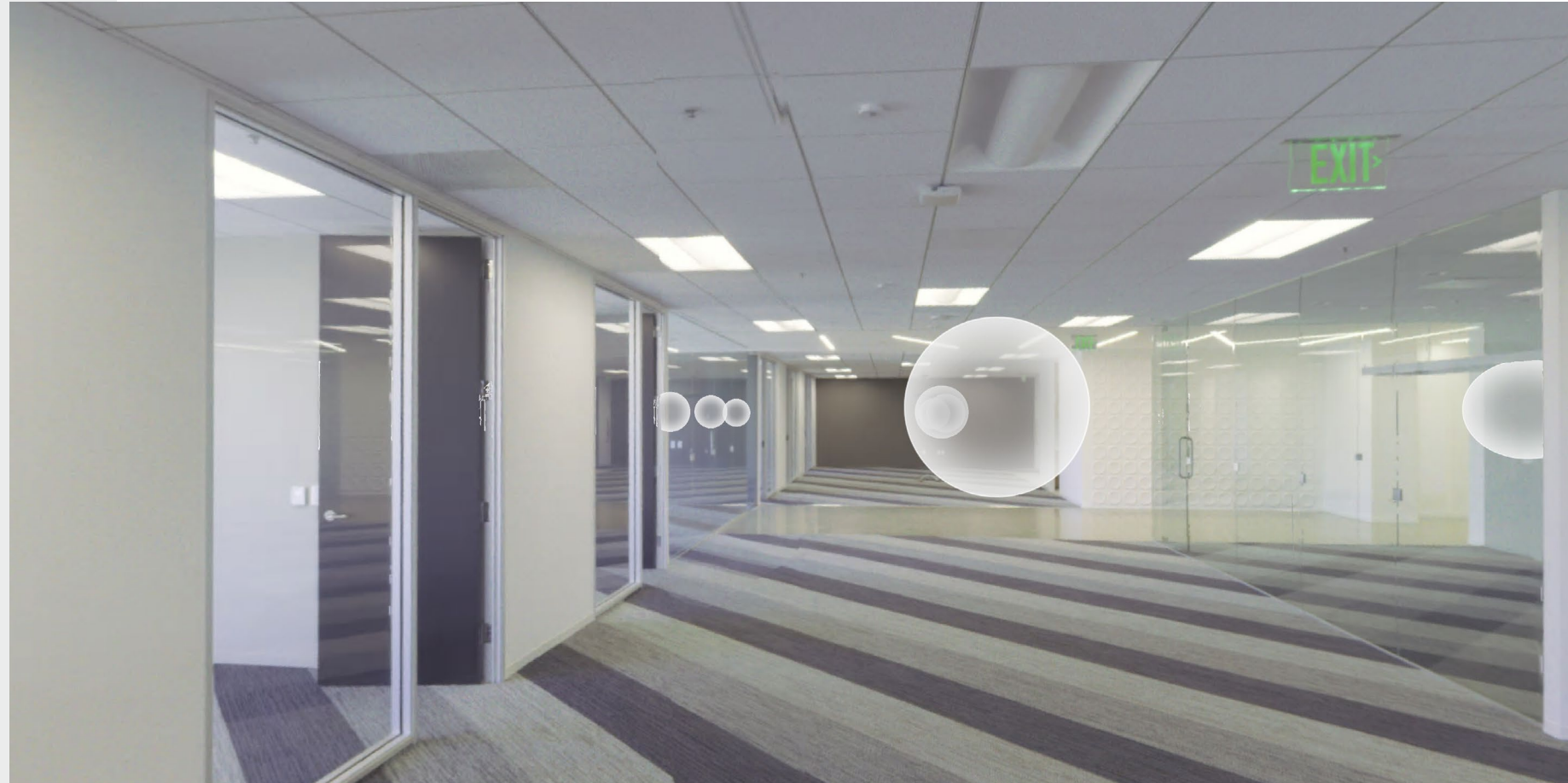
HDR image of space with white circles representing where the scanner stood.
